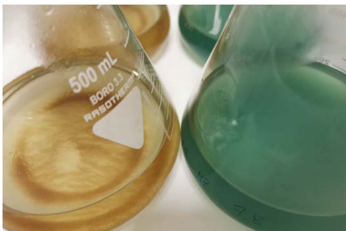
Figure 1: Control sample on the left, without decolourization and bacterial sample on the right where bacterial activity degraded lignin and decolourized the indicator in visible green color.
