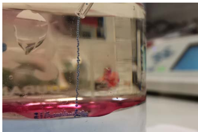
Figure 2: Alginate beads, produced by microfluidic set-up, are collected for further selection and analysis. Blue indicator is added to monitor bacterial activity of diesel degradation.
